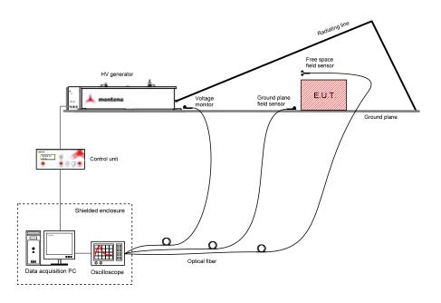
Montena systems include a range of standard size installations for EUT from a height of 50 cm up to large structures such as vehicles or airplanes. The smallest systems are transportable and can be set up and removed in less than 2 hours.
